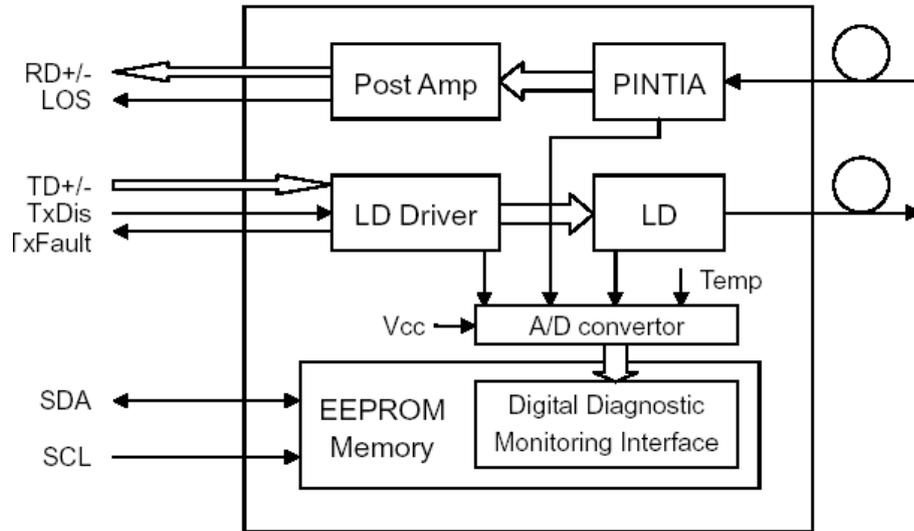
Figure 1: CCPXXD6-21-SDI Functional Block Diagram
